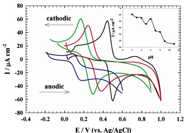
**Figure 3.** (Color online) Cyclic voltammetric response of  $1.0 \times 10^{-3}$  mol  $L^{-1}$  DA at the GNMCPe in  $0.04$  mol  $L^{-1}$  B-R buffers of different pH values [pH 2 (—), 5 (red —), 7 (green —), and 9 (blue —)]. The inset: Plot of the anodic peak current values vs pH values.
