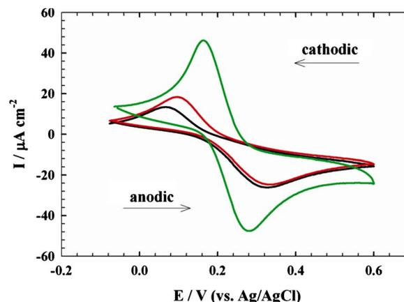
**Figure 2.** (Color online) Cyclic voltammograms of  $1.0 \times 10^{-3} \text{ mol L}^{-1}$  DA in B–R buffer pH 7.4 at a scan rate of  $100 \text{ mV s}^{-1}$  recorded at three different working electrodes: [bare CP electrode (—), AuNpCP (red —), and GNMCP (green —)].
