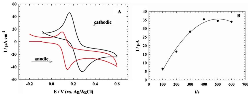
**Figure 5.** (Color online) (A) Cyclic voltammograms of  $1.0 \times 10^{-3}$  mol  $L^{-1}$  DA at the GNMCPe in different buffer types: B-R buffer pH 7.4 (—) and PBS pH 7.4 (red —). (B) Relation between the anodic peak current of  $1.0 \times 10^{-3}$  mol  $L^{-1}$  DA in  $0.04$  mol  $L^{-1}$  B-R buffer pH 7.4 at the GNMCPe and different electrodeposition times of gold nanoparticles: 100, 200, 300, 400, 500, and 600 s.
