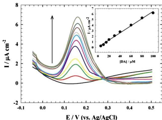
**Figure 7.** (Color online) The differential pulse voltammograms obtained at GNMCPPE for (5, 10, 15, 20, 30, 40, 50, 60, 80, and 100  $\mu\text{mol L}^{-1}$ ) DA and 0.1  $\text{mmol L}^{-1}$  UA in the presence of 5  $\text{mmol L}^{-1}$  AA in B–R buffer pH 7.4 and a scan rate of 10 mV/s. The inset shows the corresponding calibration curve of DA.
