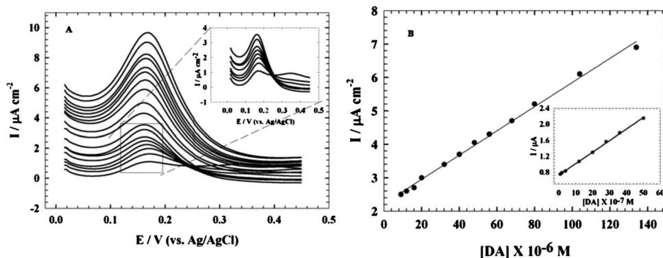
Figure 9. A The effect of changing the concentration of DA using differential pulse mode at GNMCPE in  $0.04$  mol L $^{-1}$  B-R buffer pH 7.4 and a scan rate of  $10$  mV/s. The inset represents the differential pulse mode of the smaller concentration range. (B) The calibration curve of the oxidation peak current values of  $i_{pa}$  vs the concentration of DA. The inset represents the calibration curve of the smaller concentration range.
